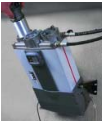
Tilt mounting kit facilitates easy cartridge replacement
