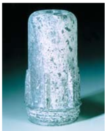
Rapid corrosion of untreated aluminium
