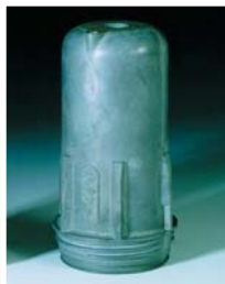
No corrosion with Alocrom treatment
