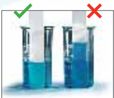
Filter media actively repels oil and water
