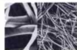
Graded density nanofiber filter media
